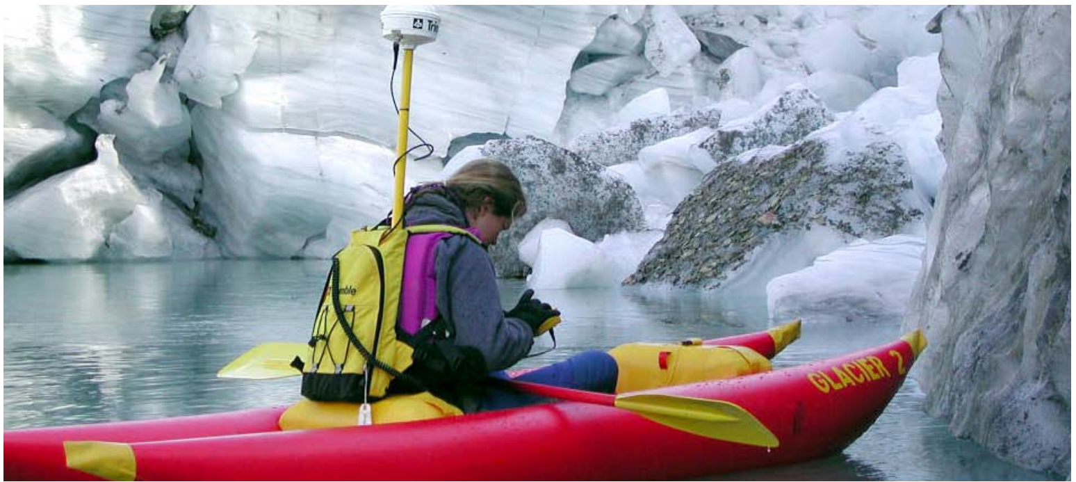
A USGS scientist collects GPS points along the terminus of Grinnell Glacier, September 2003. Photo by Lisa McKeon, USGS.
